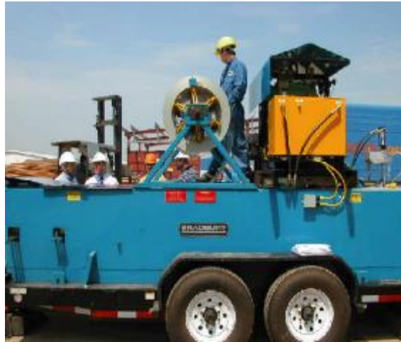
Mobile Roll Former On Site
