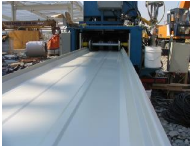
Rolling MaxSEAM® Panels On Site
